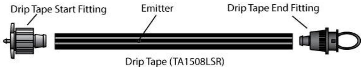
\*Some leakage may occur out of the drip tape start fittings. A quarter turn with pliers will tighten the locking collar.
