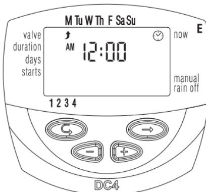
If the most recent data item stops blinking before you finish programming it, press Ⓣ to continue the programming process.
