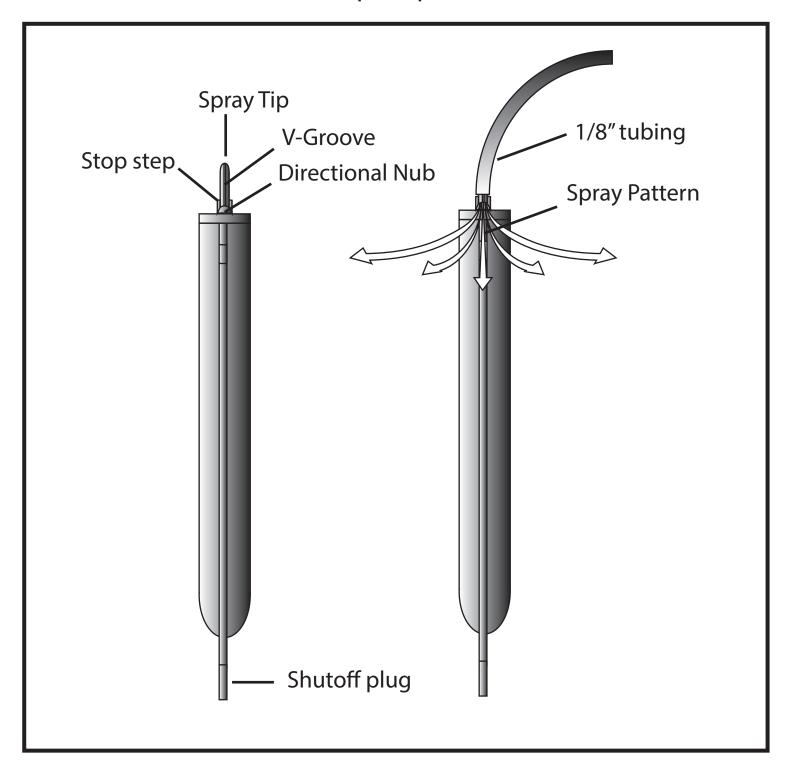
Designed for commercial container growing, these spray emitters are also great for large potted plants in residential gardens. Used with 1/8" tubing, they provide a gentle 160° cone-shaped, downward spray. Not recommended for use over 20 PSI.
