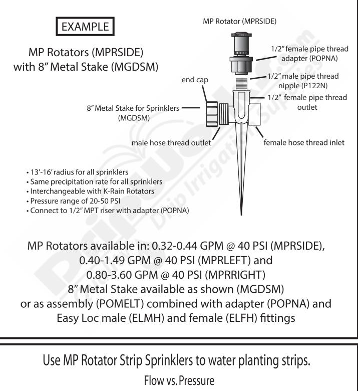
Flow is the output of water measured in GPH (gallons per hour) or GPM (gallons per minute) and pressure is the force behind the flow measured in PSI (pounds per square inch).
