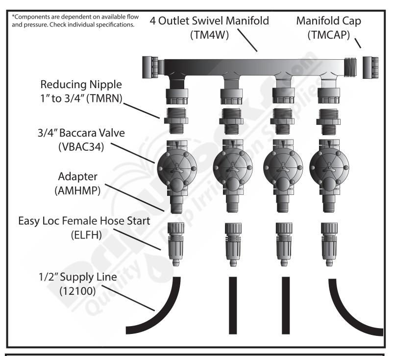
This 1" manifold assembly uses reducing nipples to connect to the inlet side of the 3/4" Baccara inline valves and adapters to transition to hose thread 1/2" Easy Loc female poly fittings.
