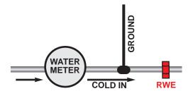
If you have a water meter, the RWE UNIT is installed on the cold water pipe, after the water meter itself, as shown. Additionally, the RWE UNIT should always be placed after any electric ground wire clamp that uses the cold water line for grounding, as shown above.
