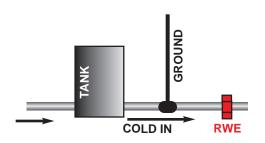
If your water is provided by a well, the RWE UNIT is installed on the cold water pipe exiting the water pressure tank. Additionally, the RWE UNIT should always be placed after any electric ground wire clamp that uses the cold water line for grounding, as shown above.
