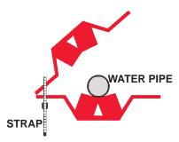
Step one: Pull strap through holes at one end of RWE unit, and loop through locking device, pulling strap almost tight.
