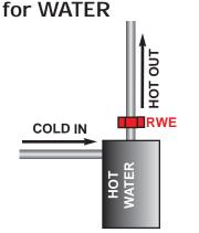
Place the RWE UNIT on the hot water pipe outlet, usually at the top of the water heater as shown above.
