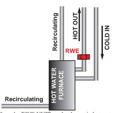
Place the RWE UNIT on the domestic hot water outlet pipe (1/2" to 3/4" pipe) as shown above. NOTE: do not place it on the heater recirculating line (1 3/4" to 2" pipe). If you are experiencing a coil blockage or restricted flow have your local plumber clean the coil.
