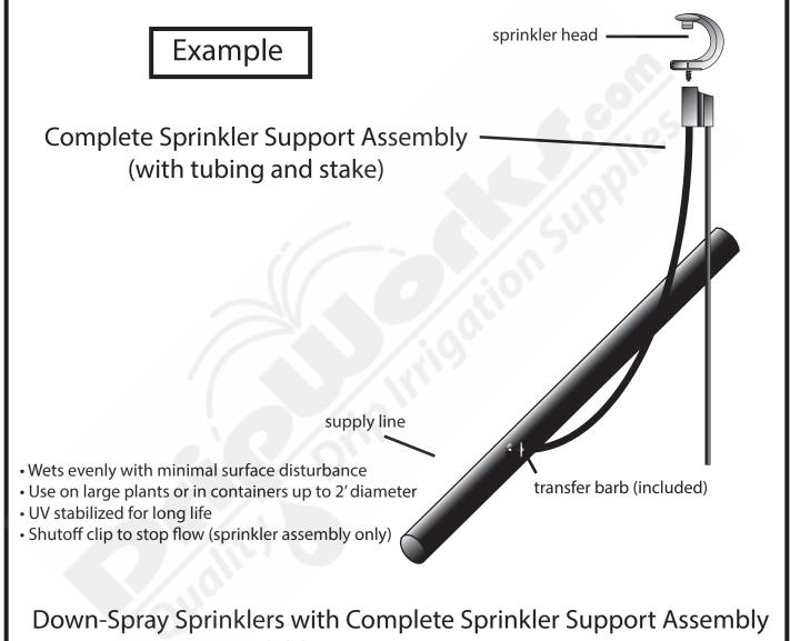
Down-Spray Sprinklers with Complete Sprinkler Support Assembly are available in: MADASBLK/MADASBLU
