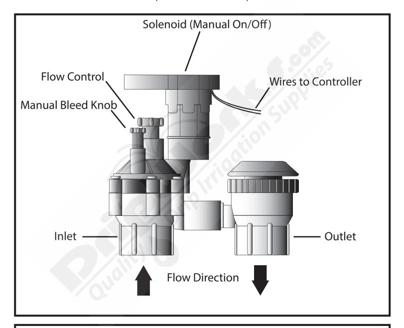
Anti-Siphon valves are designed to guard your clean water supply by preventing backflow from your irrigation system and their heavy-duty construction protects against temperature extremes and high pressure situations. To be effective, Anti-Siphon valves should be installed at least 6" above the highest point in the system and secured to a post or stake for stability.
