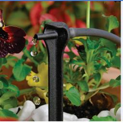
A landscape and nursery dripper incorporating an anchoring spike that delivers precise amounts of water direct to the plant root zone. This pressure compensating (PC) spike dripper has a sealed turbulent flow path and diaphragm to maintain uniform discharge rates over a wide range of pressures.
