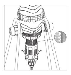
\* NOTE: If it is planned not to use the injector for a long time, it should be operated for a few minutes with the suction tube inside a tank of clean water, in order to flush away traces of additive from inside the injector and prevent them from adhering to it.
