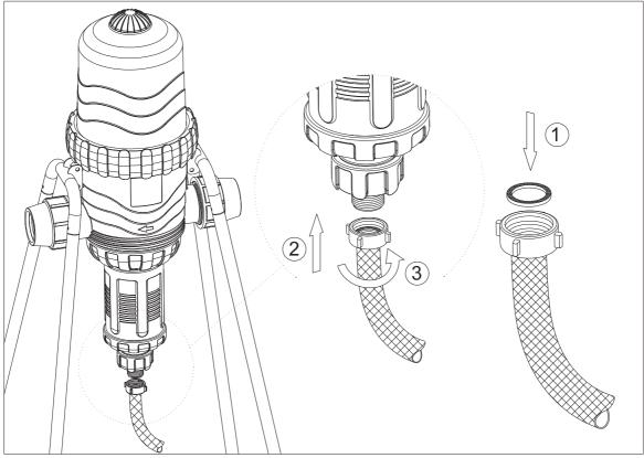
Connection of the injector to a 2" line
