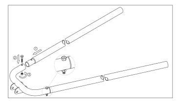
Insert the narrow part of the leg into the opening in the tube in the arched brace. Make sure that the holes in the leg are opposite the holes in the arched brace. Insert the 6mm bolt and tighten the nut. Repeat with the other legs.
